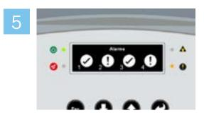
An alarm condition is initiated when smoke particles are greater than the programmed smoke alarm thresholds.
