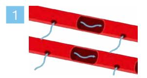
Air is drawn into the system through the sampling holes and into the aspirating pipe.
