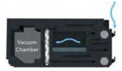
The result is the instant formation of water droplets on fire particles within the sampled air, thereby forming a cloud in the chamber.
