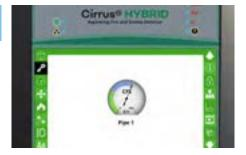
A fire condition is initiated if the fire/smoke particles are greater than the preset fire alarm thresholds.
