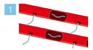
Air is drawn into the system through the sampling holes and into the aspirating pipe.
