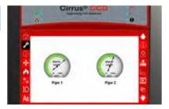
An alarm condition is initiated when combustion particles are greater than the programmed fire condition thresholds.
