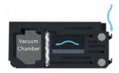
The air is drawn through the cloud chamber into a humid vacuum. The vacuum is removed. Moisture in the chamber condenses onto the fire particles, creating a cloud.
