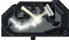
This beam is scattered onto a light receiver when visible smoke particles are present.
